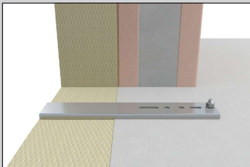
Step 3 Insert bracket into insulation. The bridges with the protection plate have to be aligned with the concrete sole. Secure it with the first Heavy-Duty Dowel.
