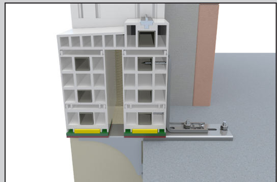
Step 4 Place second Heavy-Duty Dowel. Screw connecting angle to door element and console.
